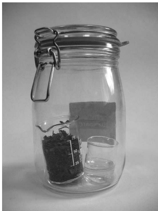
Figure 6 A simple closed respirometer—an airtight glass or plastic container with an organic matter sample and NaOH absorbing \text{CO}_2 evolved due to microbial respiration.
